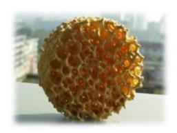
JINTAI Zirconia Ceramic Foam Filters (CFF-ZR) is available in all common sizes in the range of 40x40x20mm up to 150x150x30mm. Round filters are available from D40x20mm up to D150x30mm. Although PPI 10 is the porosity most commonly used for steel casting, finer porosities up to PPI 60 are available on request. Custom-made cut-to-size filters are also possible.
